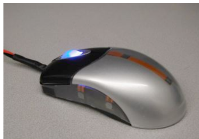
Figure 3. Pressure mouse sensor. Developed at Arizona State University based on an MIT svstem.
