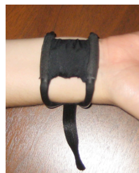
Figure 4. Conductance Bracelet A wireless skin conductance sensor manufactured through collaboration between ASU and MIT (Reynolds and Picard 2004).
